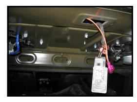
This shows the led wires coming through the factory light opening. Simply plug in the white connector into the factory light socket aligning the black wire with black and red wire with the orange/black stripe wire. Test led lights. If they don't light make sure the interior lights havent timed out or turn the socket 180 degrees as you may not have the wires lined up properly.
