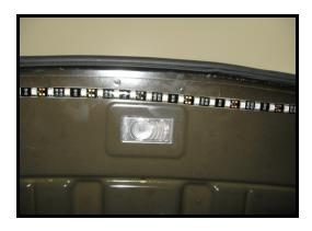
Next wipe your selected mounting area with the supplied alcohol wipe. Center the strip, peel the adhesive backing and attach the led strip in desired position. Enjoy the new lights!
