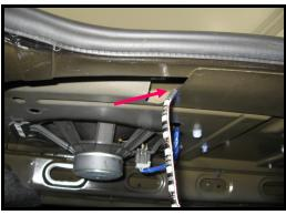
Pass the led wires through this opening and route them so they come out the factory light opening.
